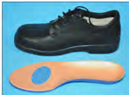
Figure 6: An extra depth diabetic shoe with an insole fitted with a PTFE patch to reduce the coefficient of friction (COF) under the second, third and fourth metatarsal heads, a common site of foot ulcerations in insensate patients.
