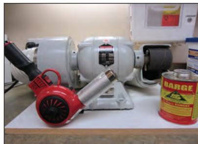
Figures 1: Orthotic modification equipment, including from left, heat gun, grinding wheel, and glue.
